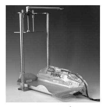
**Fig. 1:** Kraftsimulator Intra-operative Pedographie<sup>®</sup> (KIOP®). The custom made mat for force registration is covered intraoperatively with a sterile plastic bag and is placed on the KIOP<sup>®</sup>. The size of the mat is  $16 \times 32$  cm, and it contains  $32 \times 32$  sensors with a sensor size of  $0.5 \times 1$  cm.
