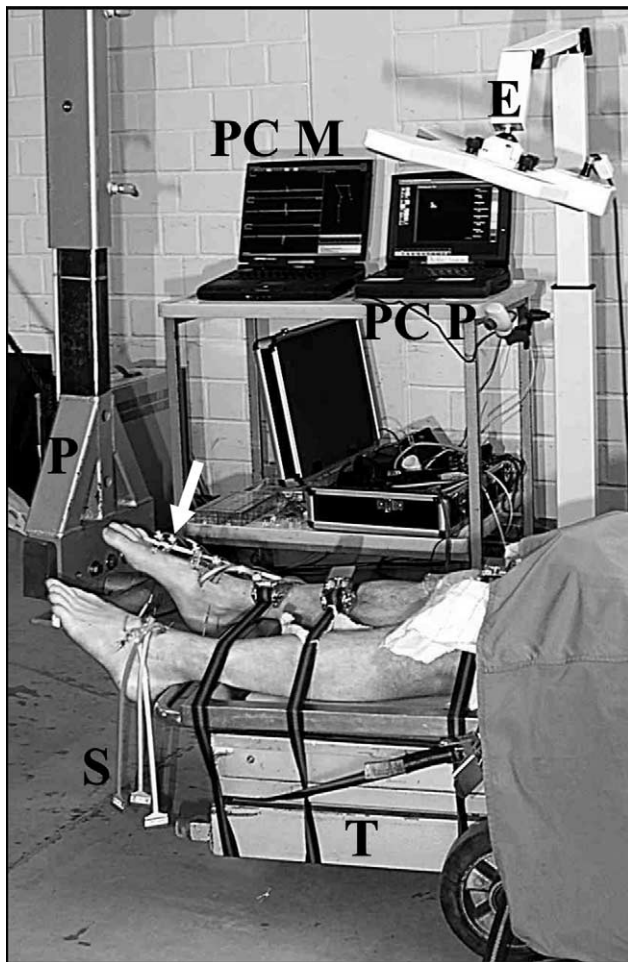
Fig. 1. Setting; P, pendulum; E, ultrasound emitter; PC P, personal computer for control of pressure measurement; PC M, personal computer for motion tracking system; white arrow, ultrasound microphone (with adaptors attached to K-wires); S, pressure sensor cables (sensors in joints); T, tray for cadaver adjustment and fixation.
