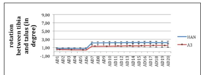
**Figure 6.** Movement in TIBTAL during the different load steps in load-to-failure testing for the HAN nail construct (plain line) and the A3 nail construct (dotted line).
