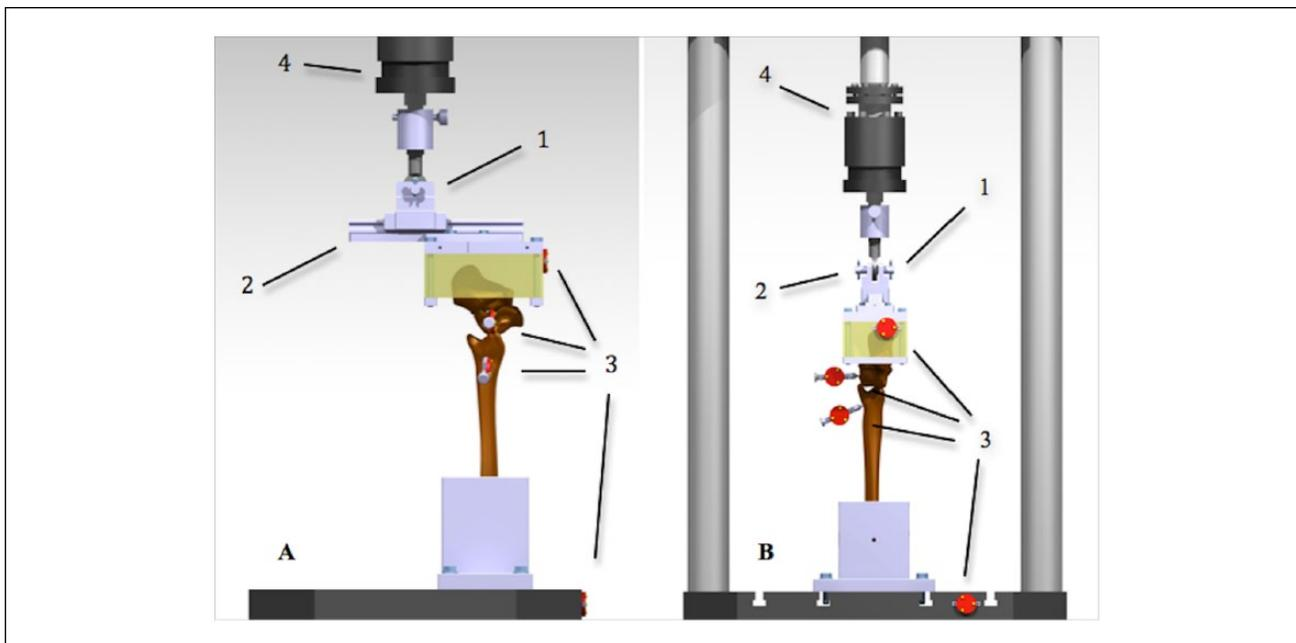
**Figure 1.** (A) Lateral view on the test setup during tests in dorsi-/plantarflexion directions, showing the embedded calcaneus linked to a slide (1) with a lever arm (2) for applying load, and the i-LEDs (3) attached to the embedded calcaneus, the talus, tibia, and the biaxial testing machine (4). (B) Anteroposterior view on the test setup.
