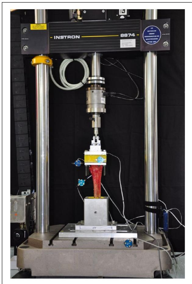
**Figure 2.** Anteroposterior view on the testing machine with an embedded specimen for quasi-static testing in dorsi-/plantarflexion directions. The i-LEDs are attached to the embedded calcaneus, the talus, tibia, and the biaxial testing machine.
