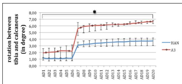
**Figure 8.** Movement in TIBCAL during different load steps in load-to-failure testing for the HAN nail construct (plain line) and the A3 nail construct (dotted line). Asterisks mark significant differences.
