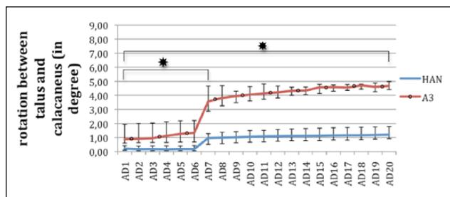
**Figure 7.** Movement in TALCAL during the different load steps in load-to-failure testing for the HAN nail construct (plain line) and the A3 nail construct (dotted line). Asterisks mark significant differences.
