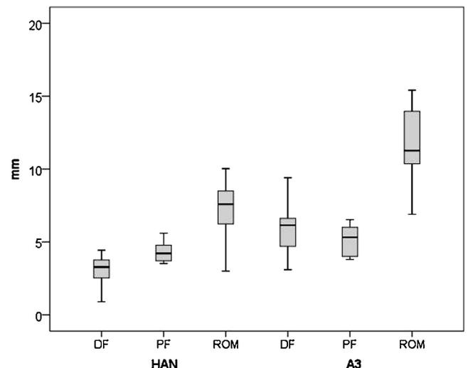
Fig. 5. Cyclic loading with 250N. Boxplots of displacement in mm. DF, dorsiflexion; PF plantiflexion; ROM, range of motion dorsiflexion–plantiflexion.
