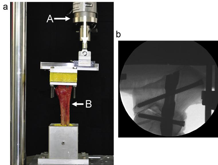
Fig. 3. (a and b) Test setting: (a) shows the test setting (A, testing machine; B, load cell; C, specimen (distal part up)) and (b) shows a fluoroscopic image.
