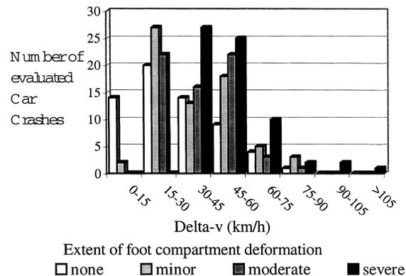
**FIG. 4.** Extent of foot compartment deformation and  $\delta v$  in 261 front seat occupants with fractures of the foot region.
