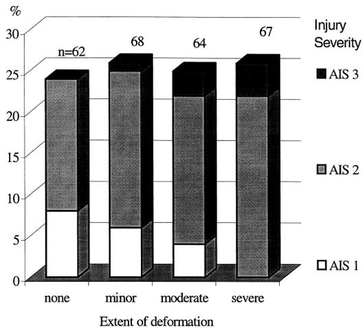
FIG. 5. Abbreviated injury scale of the foot and extent of deformation in 261 front seat occupants with fractures of the foot region.
